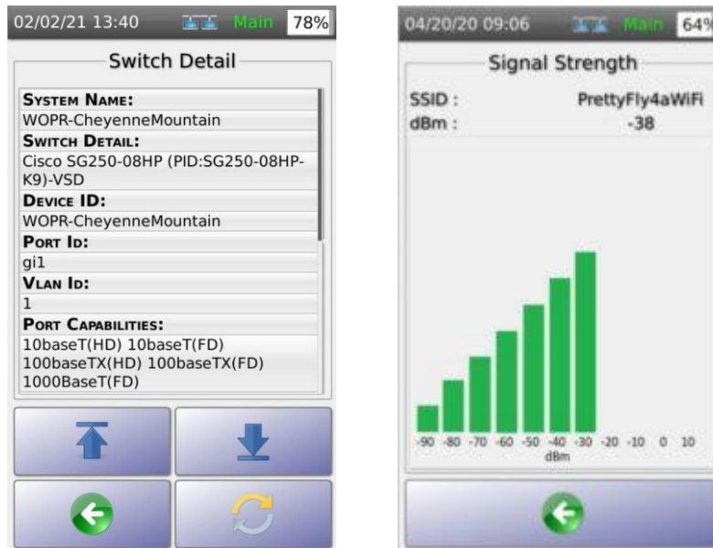
Wired switch detail and Wi-Fi signal strength verification screens
